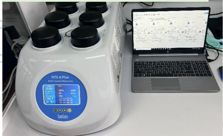
RTS-8 Plus Multi-channel bioreactor with non-invasive OD, pH and pO2 monitoring (Bio-San)
