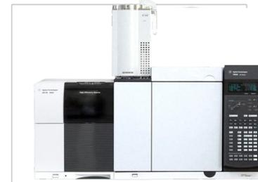
Pyrolysis-gas chromatography-mass spectrometry (Py-GC-MS)
