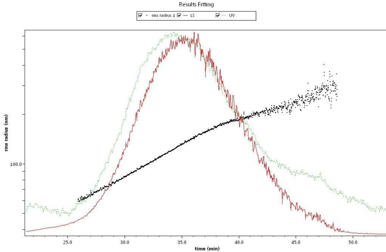
**Simple and straightforward separation of the nanoplastics after accelerated UV degradation of surgical face masks.**
