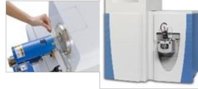
Ambient ionization-high resolution mass spectrometer DART - Thermo Q Exactive
